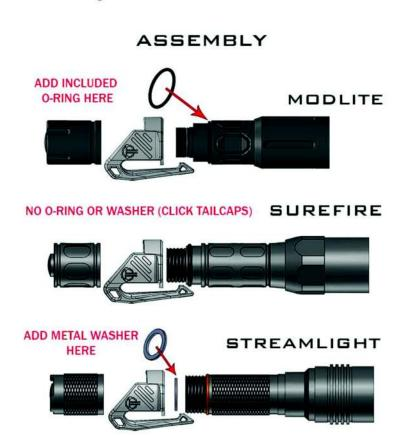
The LPC Clip installs similarly to the Thyrm SwitchBack Flashlight Ring. Leave o-ring(s) that come with your flashlight already, on the light. Unscrew the tailcap of the flashlight, then add the LPC Clip along with o-ring and/or aluminum washer before reattaching the tailcap. Note that different lights require different installation as shown in the diagram. For instance, SureFire lights with click tailcaps should need neither the o-ring nor the aluminum washer.
